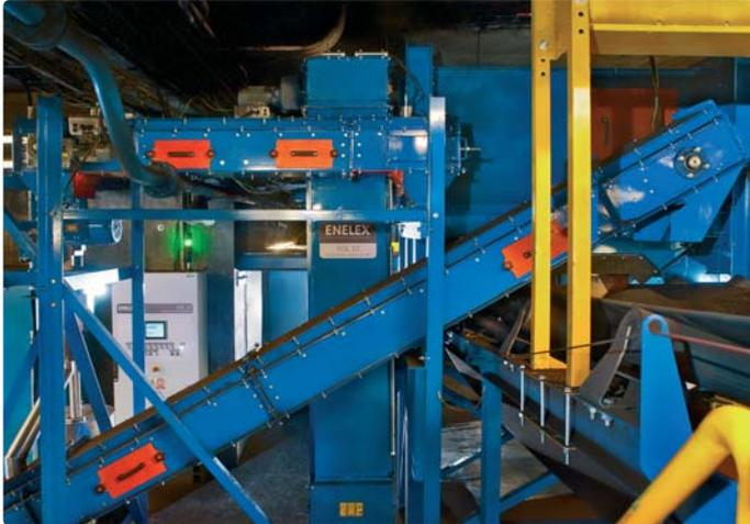
Sampling station with soft milling is fully automatic device for regular taking and sample processing from the conveyer belt using the rotary sampler. The design of the sampling device components ensures the sampling and sample processing to fully comply with required standards for solid fuels sampling.
