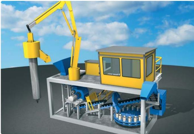
The samples are retrieved using the hydraulic boom arm with auger assembly. Unique design ensures retrieving samples from any place and any depth inside the coal trucks or rail cars using the method of submerged auger sampling, which ensures fast sampling and representative samples.
